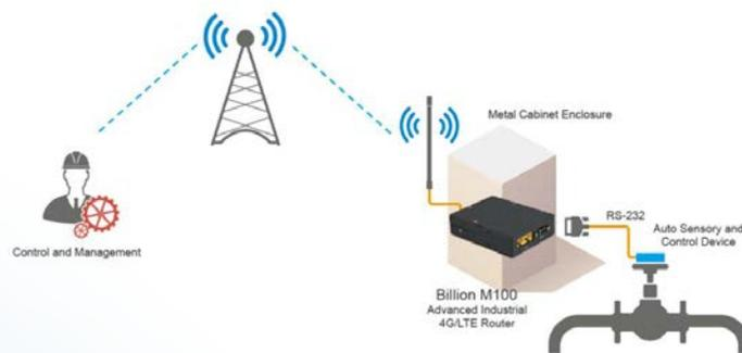
M100 supports IPSec VPN protocols to enable users to establish up to 16 VPN tunnels simultaneously in which all the data will be encrypted and transferred safely. The VPN protocol can dramatically
